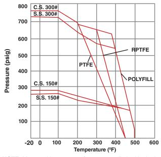
**NOTE:** Max. working pressure/temperature limited by both flange rating, seat and body seal capability.
