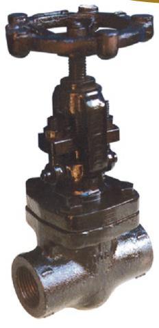
Bolted Bonnet out side screw and yoke Construction. Stem of 13% cr steel, heat treated and fine finish. Body Bonnet Gasket is fully encapsulated.
