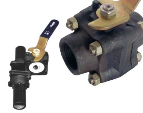
**Flowjet** Three Piece Design Ball Valves have the most easiest maintenance. To carry out any maintenance or to replace PTFE ring set, just remove three bolts and loose the forth one, the body part will Swung away. This is extremely advantageous as the valve does not have to be removed out of the line.
